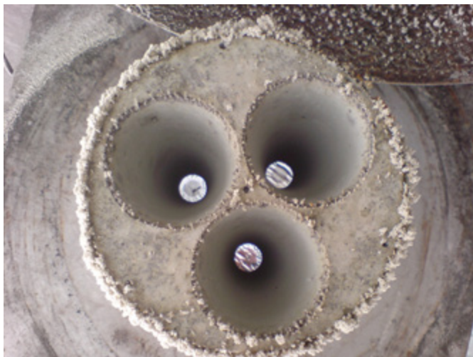
The outside of the sensor is coated with dust. Inside the transducers are clean and fully operational.
