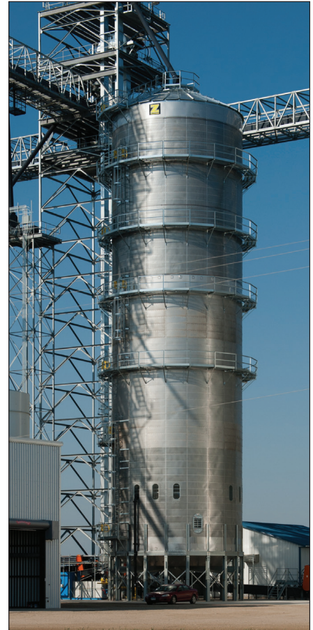
A Zimmerman grain dryer has a capacity of 10,000 bph per five points of moisture removal and is fueled by propane.
