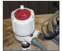
The SmartBob2 (top) and a high level capacitance probe.
