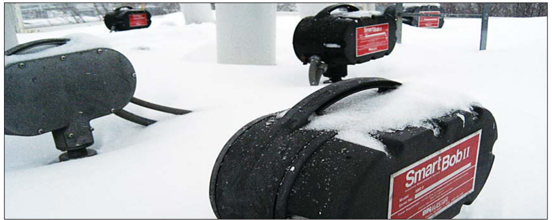
SmartBob2 level sensors measuring grain in outdoor storage silos.
