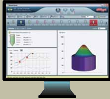
3DLevelScanners: Two or more may be installed in wide bins to cover more of the material surface. Data from the sensors is combined to provide a single visualization.
