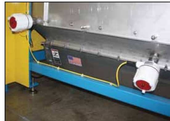
Multiple capacitance probes can be used in a single vessel.
