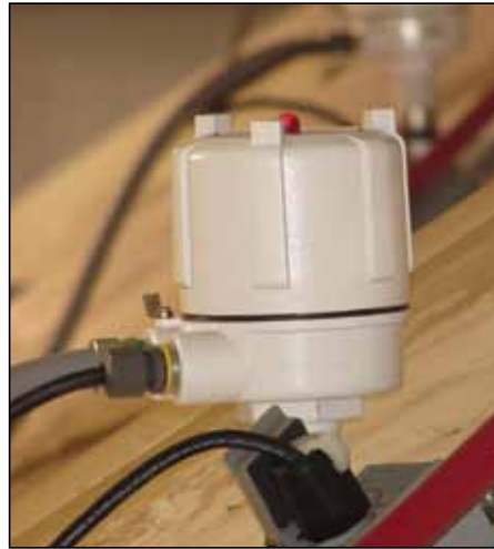
Capacitance probes are a versatile point level indicator.
