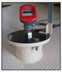
Scanner mounted on existing flange. using an adapter plate.
