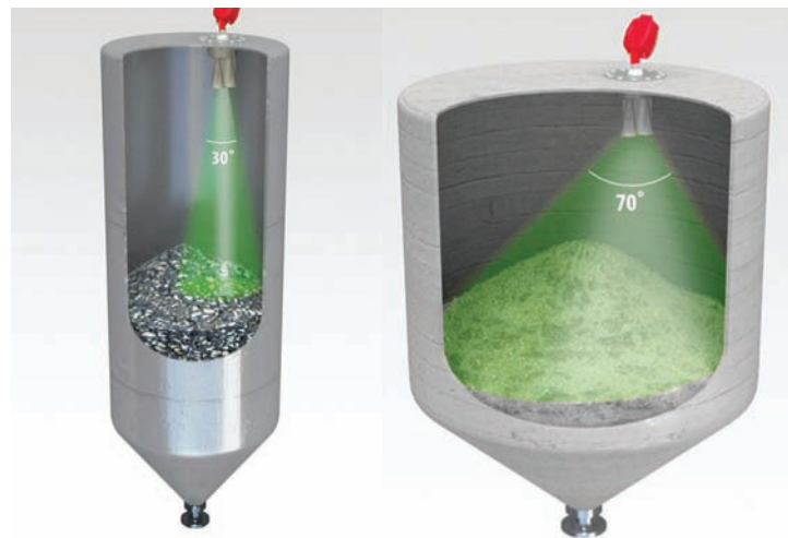
The S model (left) measures multiple points within a 30°-beam angle and is ideal for smaller silos. For larger silos, the M model (right) measures multiple points within a 70°-beam angle to accurately calculate volume.
