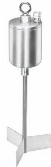
A tilt switch point level device sends an alert when material reaches the switch and tilts it 15°.
